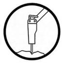
The correct pressure (A). An insufficient pressure would cause vibrations to the machine and breaker's energy would not be completely released on the boulder.
