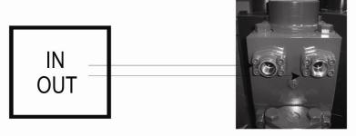
The hose is connected to the breaker using nipples 1"GAS M-M.
