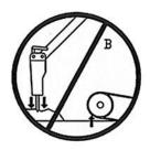
Do not insist on the same point. Do not beat on the same point for more than 30 consecutive seconds; if you can not break within this time period, change the position into parallel trying to break a smaller section. Doing so will prevent the overheating of the tool and of the whole breaker by induction
