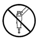
**Correct Position.** The breaker can work at any angle. However it is important that the boost is always given along the axis of the tool of the breaker.
