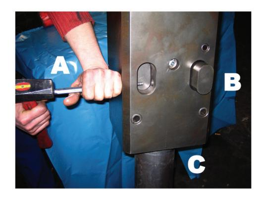
WARNING: IT IS IMPORTANT TO PLACE THE CYLINDRICAL PIN BY FIRST AND THEN THE ELASTIC PIN.
