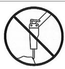
**Blank Firing.** Special care has to be taken not to carry out blank firing. A blank firing may cause Tie Rods' breaking. These are parts which keep together the various components of the breaker. Furthermore it may cause Retaining Pins' and Tools' breaking. Thus you have to disconnect the power supply to hammer at the exact moment of rock breaking.
